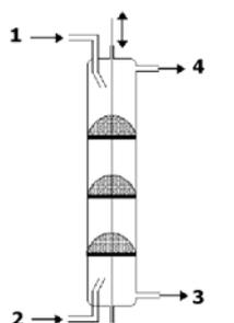
Figure 1. Extraction micro-column with pulsed caps: (1) Pineapple juice inlet (continuous phase); (2) Micellar solution inlet (dispersed); (3) Heavy phase outlet (extracted); (4) Light phase outlet (raffinated).
